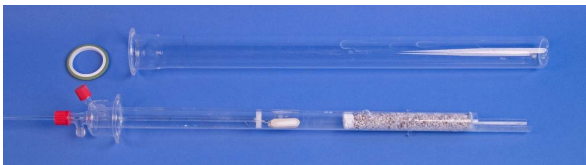
227 228 Figure 2: Glass reactor filled with \text{SrO} with additional \text{HCl} source
